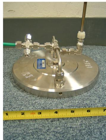
We can also test *in situ* the emission rates from flooring and other materials using the Field Laboratory Emission Cell (FLEC), see photo above on right.
