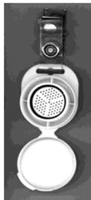
Passive formaldehyde sampler with fiberglass coated DNPH with HPLC analyses provides a reporting limit of 0.003 ppm (3 ppb, 4  $\mu\text{g}/\text{m}^3$ ) for a 24-hour sample.
